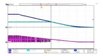
Figure 12. SCT2320 Switching Node Waveform
