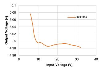
Figure 10. Line Regulation (IOUT=2A)
