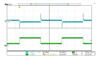
Figure 20. Load Transient VOUT=5V, IOUT=0.5A to 1.5A, SR=250mA/us
