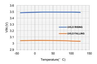
Figure 8. VIN UVLO vs Temperature
