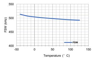
Figure 6. Center Switching Frequency vs Temperature
