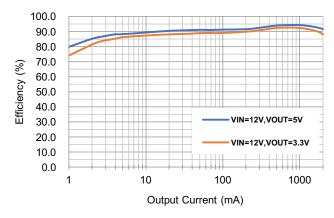
Figure 1. SCT2320 Efficiency, Vin=12V
