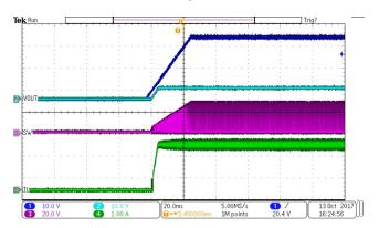
Figure 17. Power Up VIN=24V, VOUT=5V, IOUT=2A
