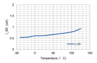
Figure 3. Shut-down Current vs Temperature
