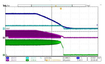
Figure 18. Power Down VIN=24V, VOUT=5V, IOUT=2A
