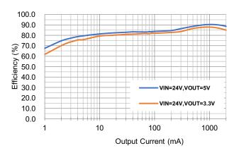
Figure 2. SCT2320 Efficiency, Vin=24V
