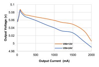
Figure 9. Load Regulation (VOUT=5V)
