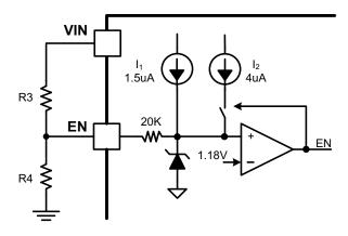
Figure 11. Adjustable VIN UVLO
