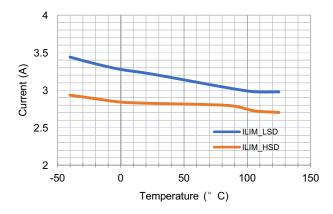
Figure 7. Peak Current Limit vs Temperature
