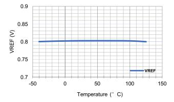
Figure 5. Reference Voltage vs Temperature
